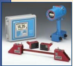
Easily installed without cutting pipe or stopping flow, these meters provide extremely accurate Wide Beam Transit-Time ultrasonic flowmetering. Suitable for essentially any liquid, and capable of operating even under high aeration conditions that usually require less accurate Doppler flowmeters.
