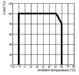
For UL and CSA the maximum temperature is 50% (with derating of  $2\%/^{\circ}C$  from 40 °C to 50 °C, only for 40 A model)
