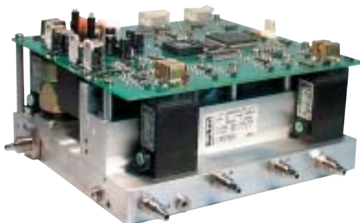
Highly integrated systems: Gas flow control unit
