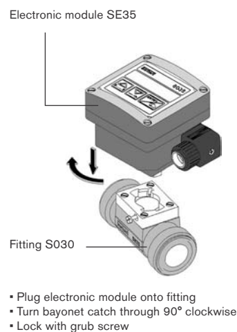
Installation of an Inline sensor using Type 8035 as an example
